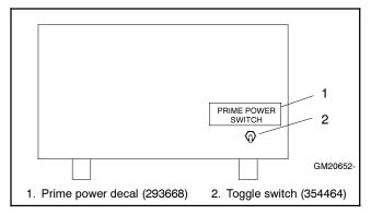
Figure 6-12 Prime Power Switch Installation Location
